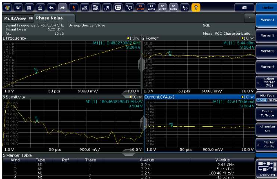
A typical VCO measurement. Key parameters such as frequency, power, sensitivity (tuning slope) and current consumption are measured relative to the tuning voltage.
